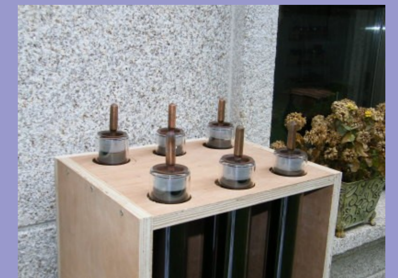
heat pipes condensers
