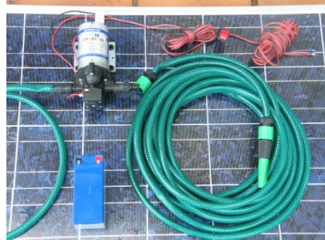
Figure 4. The solar pumping set
