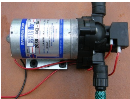
Figure 3. Shurflo 2088 water pump
